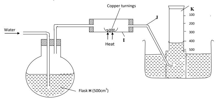
A 500cm<sup>3</sup> measuring cylinder **K** was filled with water and assembled for gas collection. Copper turnings were heated red hot and water was slowly passed into 500cm<sup>3</sup> flask **H** until it reached the 500cm<sup>3</sup> mark. A colourless gas was collected in **K**.
