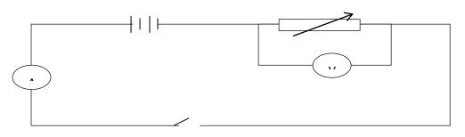
b) Adjust the potentiometer until you are able to obtain minimum reading on the voltmeter and maximum on the ammeter. Record these readings in the table below.
