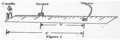
(g) Put the object at a distance u = 30cm from the mirror. Adjust the position of the screen until a sharp image is formed
