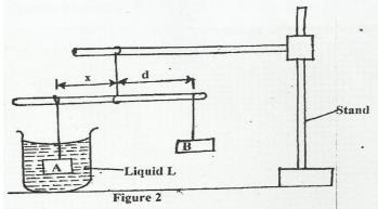
Suspend the sums A at a distance x = 50mm. adjust the position of mass B until it balances mass A immersed in liquid
