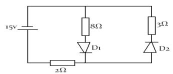
i). Calculate the current flowing through the  $2\Omega$  resistor.
