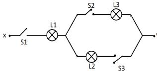
i). Other than L<sub>1</sub>, state the lamp that will light when S1 and S<sub>2</sub> are closed.
