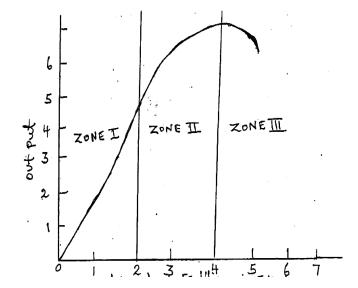
Zone marked I: output /product increases at increasing rate; under utilization of resources
