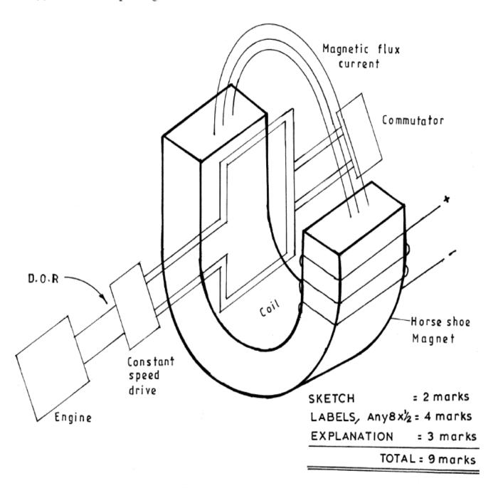
The aircraft engine rotates through a constant speed and drives a coil placed in a strong magnetic field.
