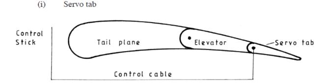
This is the type of tab that is connected to the main control stick to raise or lower the aircraft nose.
