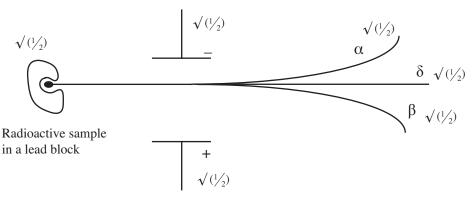
Working diagram,  $\alpha$  should be deflected less than  $\beta$  because of its heavier mass.
