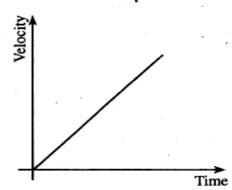
(straight line not necessarily through the origin but with positive gradient) acceleration; constant acceleration;
