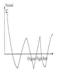
When an aircraft is disturbed by a force e.g. gust and it is withdrawn the aircraft oscillates with the amplitude remaining constant. Although this type of stability wont be disastrous, it is not comfortable to the passengers.
