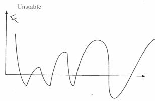
When an aircraft is disturbed by a force and the force is withdrawn, the aircraft oscillates and the amplitude of the oscillations increases in magnitude and can easily lead to a disaster.
