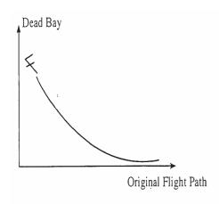
When an aircraft is disturbed by a force e.g. a gust and it is withdrawn the aircraft goes back to its original flight path without any oscilations.
