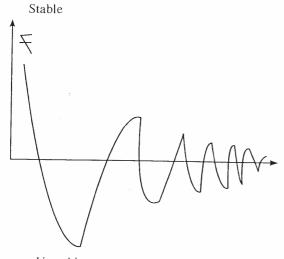
When an aircraft is disturbed by a force and the force is withdrawn, the aircraft oscillates but the oscillators are gradually dampened out.
