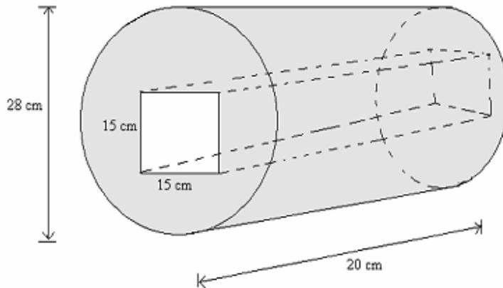
$$\begin{aligned} \text{Volume of solid} &= \text{volume of a cylinder} - \text{volume of the square hole} \\ &= \left(\frac{22}{7} \times 14 \times 14 \times 20\right) - (15 \times 15 \times 20) \\ &= 12320 - 4500 \\ &= 7,820 \text{ cm}^3 \end{aligned}$$
