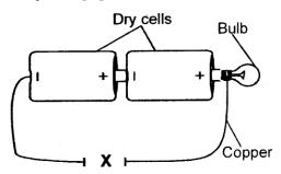
Which one of the following materials when placed at part X will NOT make the bulb light?
