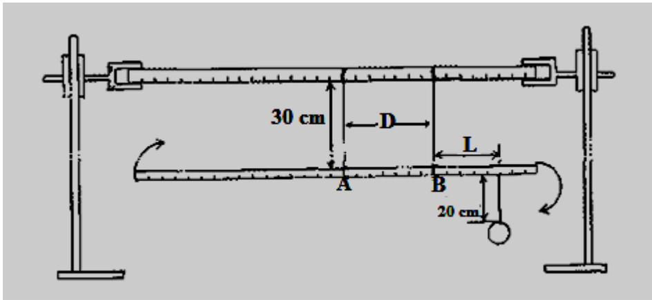
Starting with a distance  $D = 15\text{cm}$ , and distance  $L = 25\text{ cm}$ . displace the hanging metre rule on a horizontal plane and record the time taken for it to make 20 complete oscillations on table 1.
