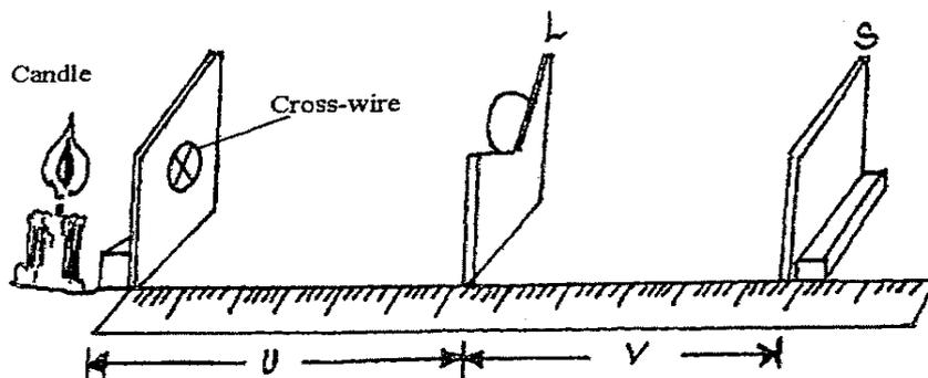
(c) Starting with  $u=30\text{cm}$ , vary the position of the screen S until a sharp image of the cross wire is observed on the screen. Measure and record the value of the image distance  $v$ .
