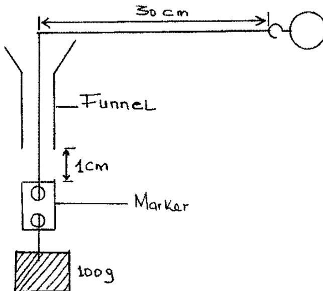
i) Hold the funnel vertically. Swing the pendulum ball around so that it moves in a constant horizontal circle with a uniform circular motion. The marker should be just below the funnel but not touching it. Measure the time taken by the Pendulum ball to make 10 complete revolutions and repeat this 3 times and complete the table below. (3mks)
