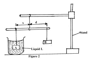
Suspend the mass A at a distance x = 50mm. adjust the position of mass B until it balances mass A immersed in liquid L.
