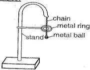
When cooled the metal ball will pass through the ring. When heated the metal ball did not pass through the ring. What would happen when the ball and the ring were heated at the same time under same temperature?
